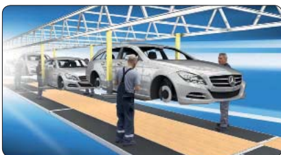
The Personnel Transfer System
